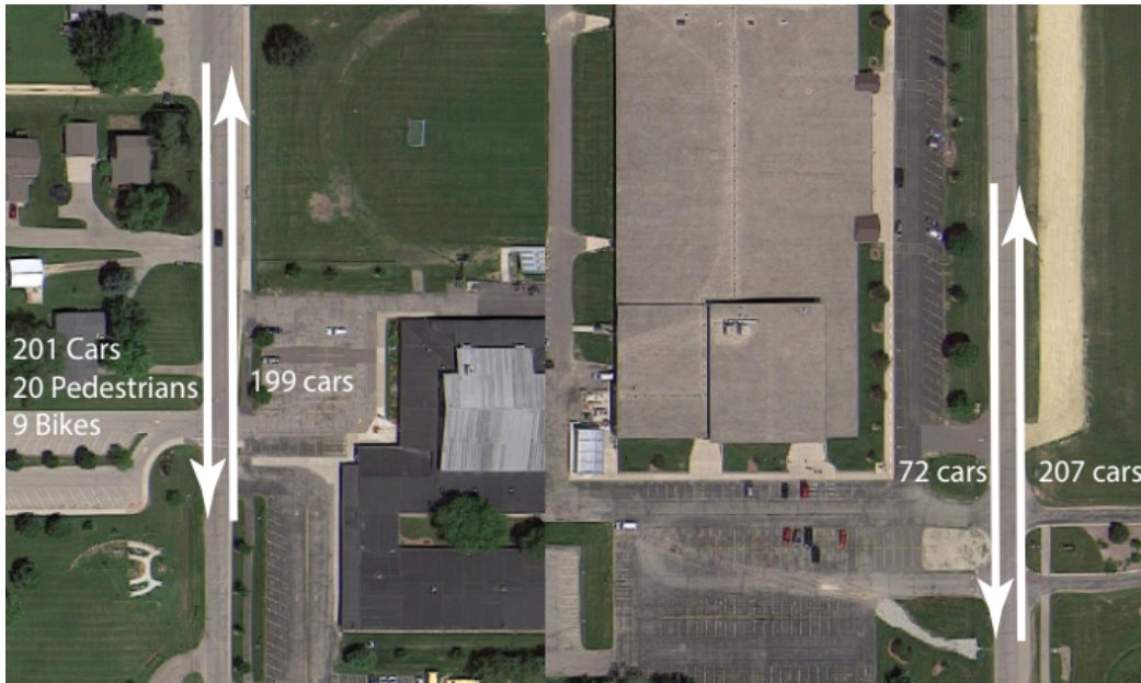
Figure 3. Total traffic counts for the ES (left) and HS/MS (right) during AM drop-off times.
